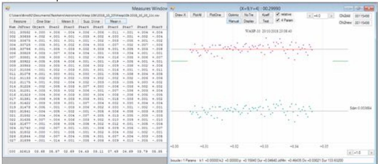
D- QHY 42C 24x(30x2sec) : stdev = stdev=1.16/1000 (This means that for a 12 mag star, it is possible to get a millimag error on 60 seconds images).
