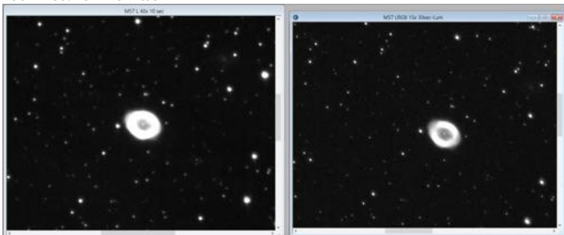
Number of ADU on a 12 pixel aperture radius : QHY42 : 437.000 ADU (12bits) for 10 seconds (left), FLI : 134.000 for 30 seconds (right); ratio QHY42/FLI = 9.8 (surface)
