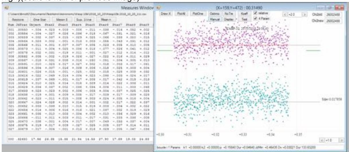
C- QHY 42C 24 x (9 x 2 sec) : stdev= 3.7 / 1000 (this means that an 18 seconds shot with the QHY42c is equivalent to a 60 seconds shot with FLI11002)
